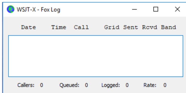
13. To send logged QSOs directly to *N1MM Logger+*, go to **Settings | Reporting**, check **Enable logged contact ADIF broadcast**, and enter the IP address and port number used by your N1MM server.
